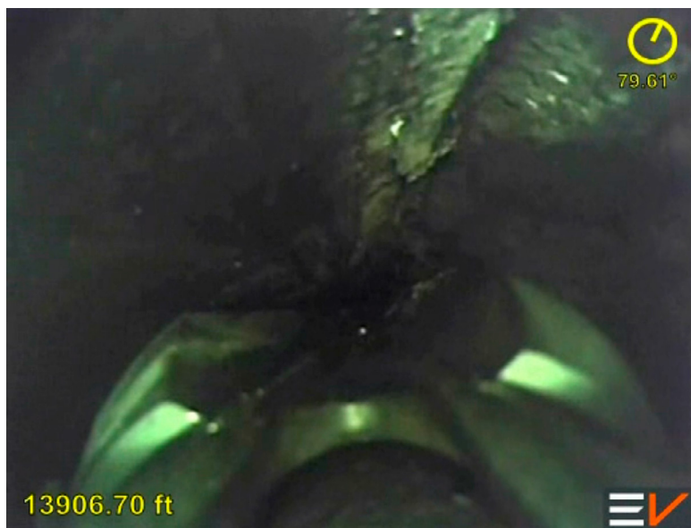
Figure 1: Confirmation of completion window misalignment
