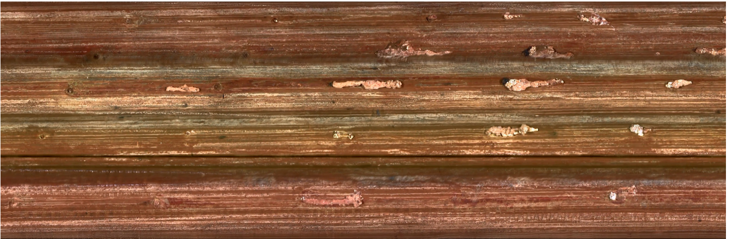
Figure 2: 360 degree mosaic image of plugged perforations
