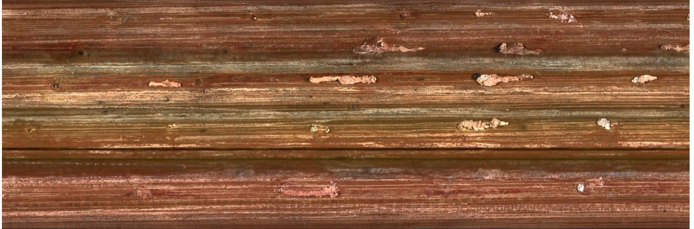
Figure 2: 360 degree mosaic image of plugged perforations
