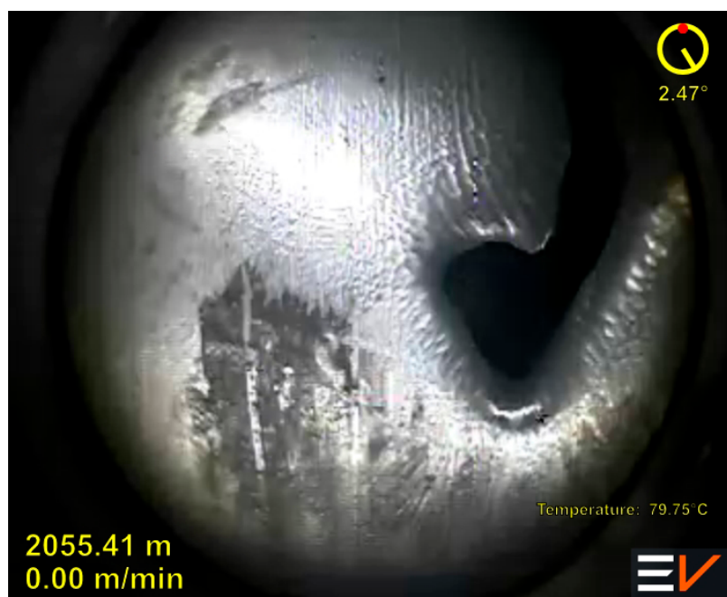
Figure 1: Sideview footage of casing breach
