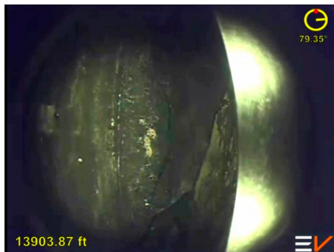
Figure 2: Sideview image of casing overlap
