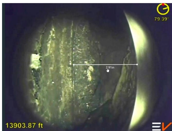
Figure 3: Measurements confirming extent of casing overlap
