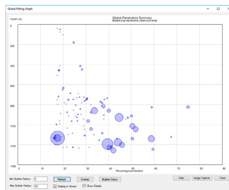
Global analysis allows the user to find the largest wall penetrations, cluster neighbouring penetrations, and show the relative size of the clusters in a summary graph. Overlays can be used to compare passes and for time lapse analysis.
